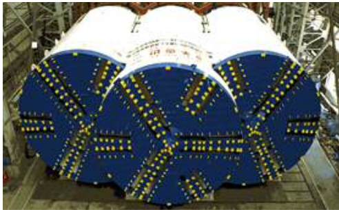
Figure 3. TBM with 3 faces used the construction of Osaka Business Park station in line-7. Figure 4. TBM with rectangular face used in Kyoto.
