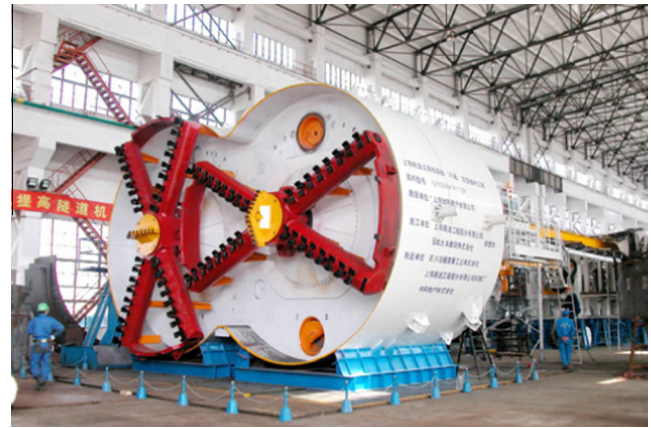
Fig. 2. DOT machine used in the construction of the Shanghai Metro.
