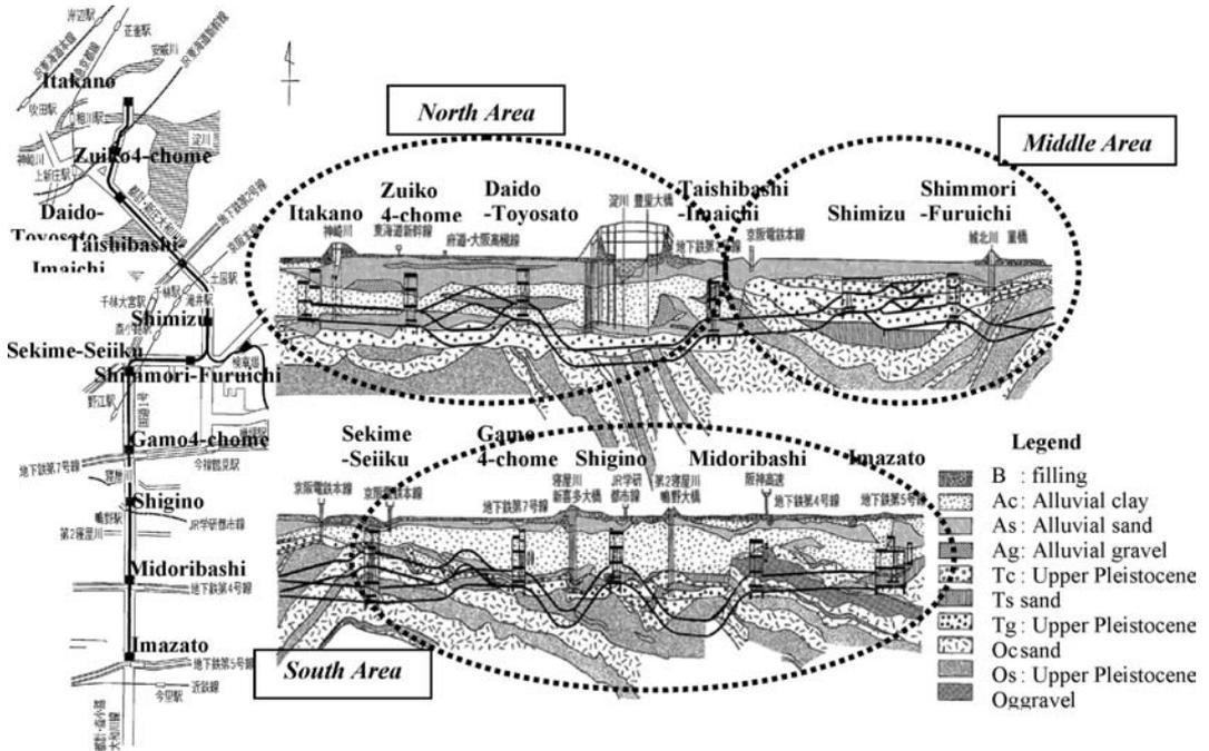
Figure 1. Plain view and soil crossing view of Osaka Subway Line No. 8 (Unei *et al.*, 2002).
