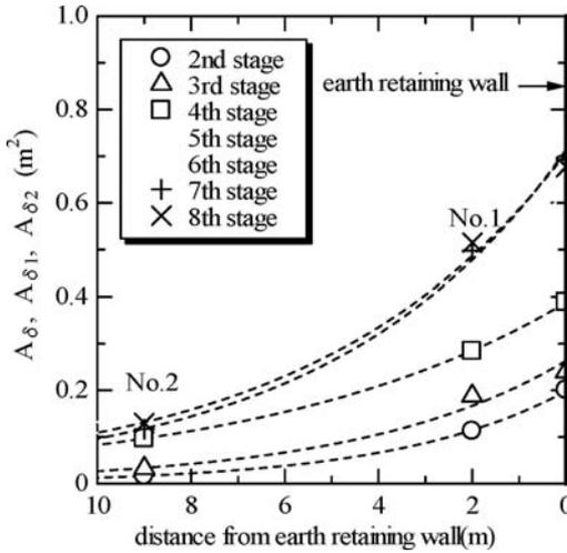
Figure 7. Influence propagation aspect to backside ground due to braced excavation.
