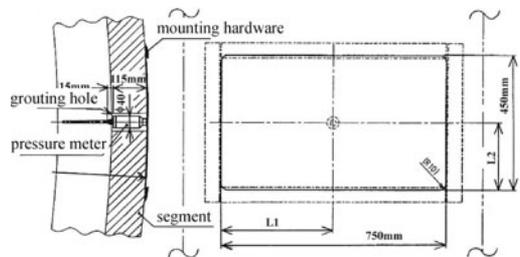
Figure 2. Pad type earth pressure cell.
