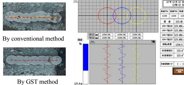
Figure 12. Verticality control system of GST method.
