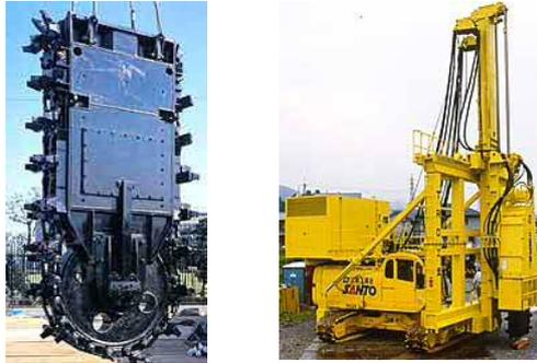
Figure 11. TRD method machine.
