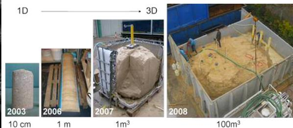
Figure 18. Development of improvement soil by BioGrouting.
