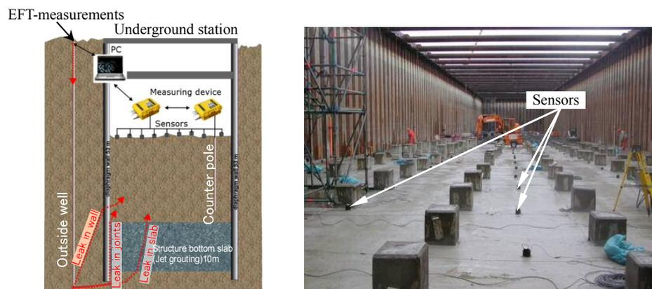
Figure 2. Scheme of leaks detection by ECR/EFT.
