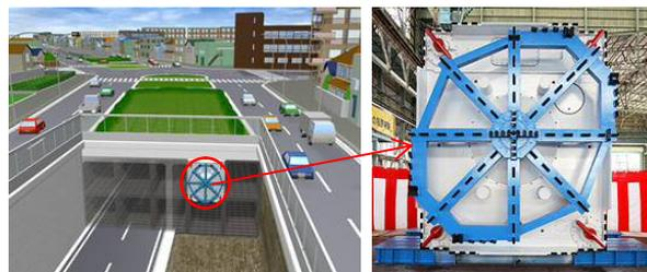
Figure 10. Harmonica Tunneling Method.
