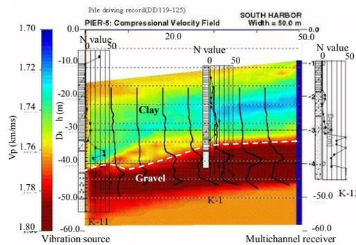
Figure 1. A velocity imaging of acoustic wave tomography.
