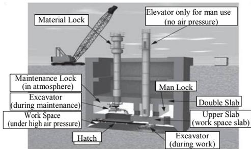
Figure 13. The Remote controlled Pneumatic Caisson.
