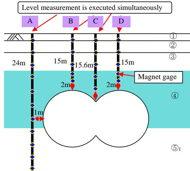
Fig.2 Instrumentation of monitoring section
